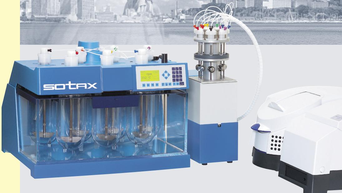
**The SOTAX AT 7smart on-line automated dissolution system with the Evolution 300 spectrophotometer from the Thermo Electron Corporation:**
